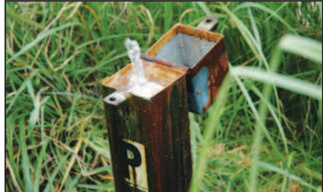
Above, Water table elevation monitoring well spewing groundwater. Below, the stream begins to rise from the water pressure. Photo provided by CALH.
